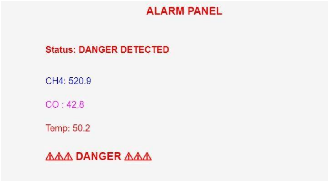
Figure 5.1 Robot mission alarm panel indicating detected hazardous conditions
